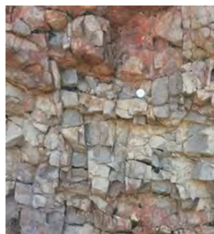
Below Right: Park Limestone Formation being worked at Sandside Quarry. A distinct fault is shown in the middle of the photograph, around which extraction of the rock is more difficult
