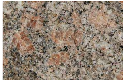
Detail of Shap Granite showing large, interlocking crystal structure
