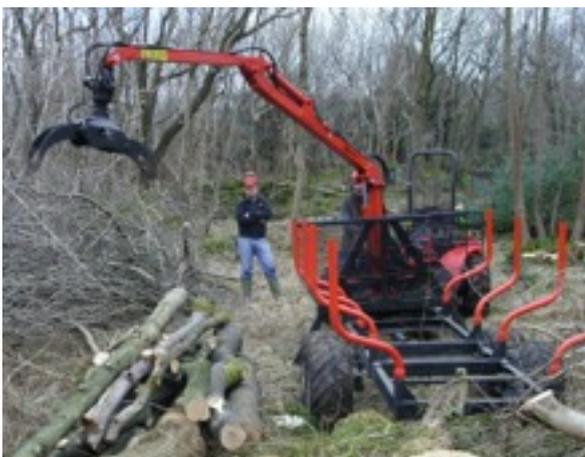
Narrow and lightweight, the compact tractor with winch and timber trailer can negotiate small gateways, large rocks, stumps and brash. Depending on the site, the tractor can work from where the timber is felled with the winch and can also quickly move long length logs to the edge or out of the woodland. Three-tonne capacity.
